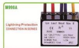
Uc:120-277VAC Up: 1200V In(8/20):5kA Imax(8/20)10kA Surge Protection Voltage:10kV CE RoHS
