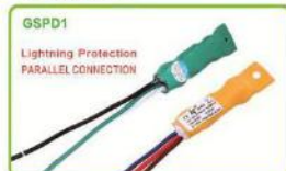
Uc:120-277VAC Up: 850V In(8/20):10kA Imax:20kA Surge Protection Voltage:10kV CE RoHS
