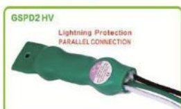
Uc:347-480VAC Up: 1355V In(8/20):12kA Imax:24kA Surge Protection Voltage:20kV CE RoHS
