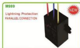
Uc:277VAC Up: 1200V In(8/20):6kA Imax(8/20)10kA Surge Protection Voltage:10kV CE RoHS
