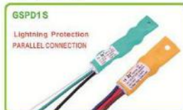
Uc:120-277VAC Up: 850V In(8/20):5kA Imax:10kA Surge Protection Voltage:10kV CE RoHS
