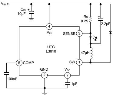
4.5~40V input voltage, 350mA output LED driver
